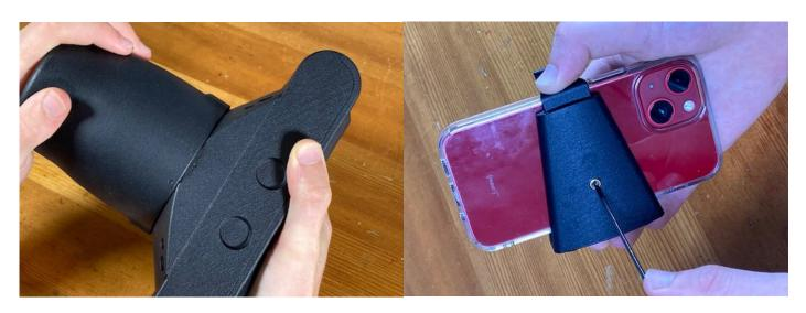
Rotate lens cover anti-clockwise to remove. Align dots and turn clockwise to attach.
